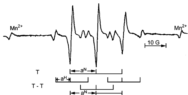
Figure 13. ESR spectrum observed at room temperature for a PMMA–benzene solution with added PMNB after 2 h of ultrasonic irradiation at 40 °C. Stick diagrams are also shown in which a^H and a^N (the hyperfine coupling constants) stand for separations due to coupling of the radical to a hydrogen and nitrogen nucleus. 178
