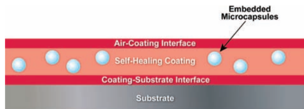
Figure 54. Schematic of a microcapsule-containing self-healing coating and interfaces affected by mechanical damage. 435
